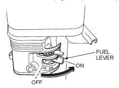
Figure 11. Fuel Valve Lever
